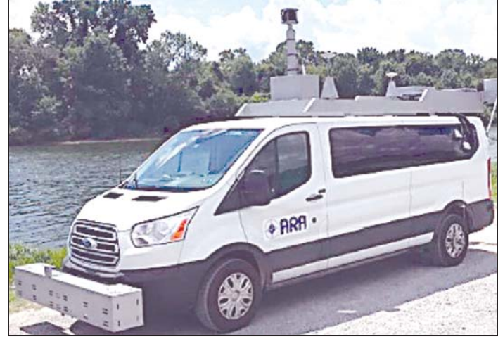
RESIDENTS IN DIAMOND and Wilmington will see a specially outfitted van driving its streets next week. The digital survey vehicle will be capturing road data the towns can use to develop a pavement management plan. The cost of the survey is being covered through a grant received from the Chicago Metropolitan Agency for Planning.
